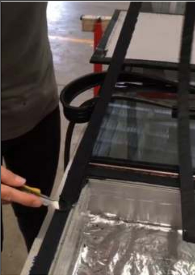
Deglazing of curtainwall panel in accordance with sealant and customer requirements
